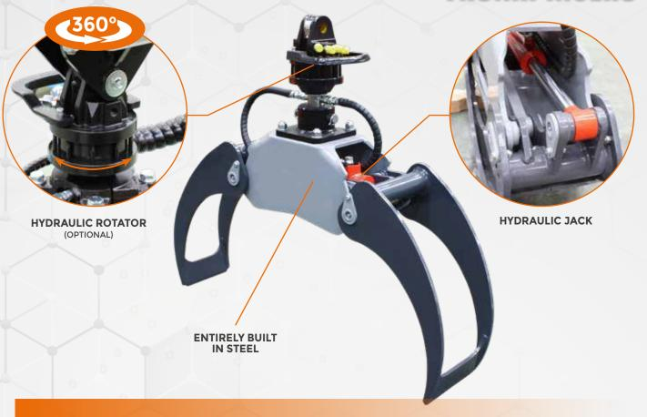
TRUNK PINCERS is an agroforestry for gripper handling tree trunks. It offers an optimal grip of the load, through the particular geometry, designed to give a closing force superior to the standard. It is made of high strength and flexible materials to allow a quick and safe grip of the material to be moved. It has pins with internal lubrication.
