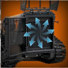
RoboMIDI is equipped with the self-cleaning reversible fan FLEXXAIRE<sup>®,</sup> to increase productivity and fuel saving.
