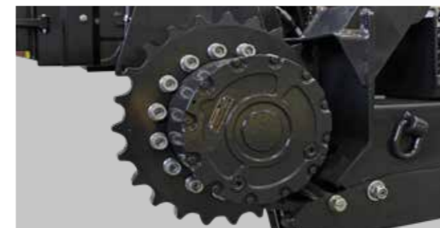
Cogwheel of the tracks in tempered steel
