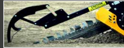
Steel Crumb with loaded spring to permit a correct trench operation and safe time to work
