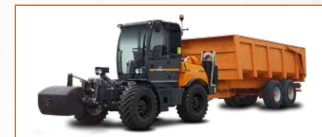
TOW KIT WITH HYDRAULIC BRAKING 10 T.
