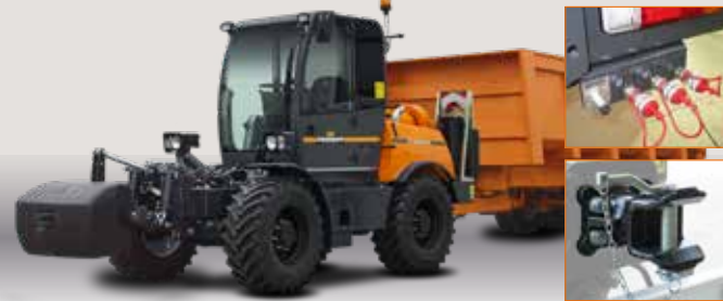
Hydraulic braking (10 T) OPTIONAL
