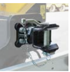
TOW KIT WITH HYDRAULIC BRAKING 10 T.
