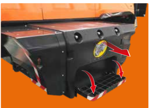
Moving ballast with step
