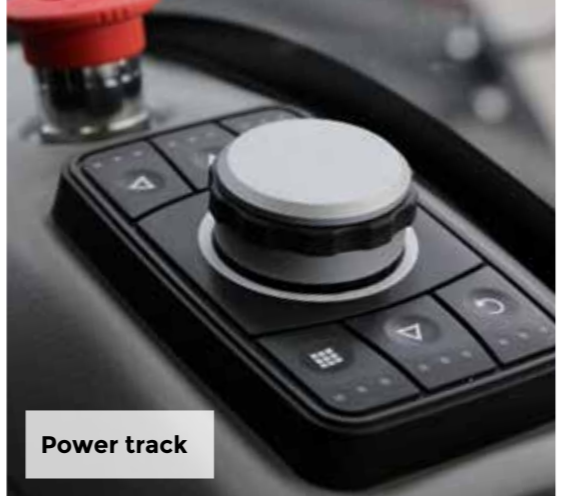
Proportional distributor Joystick
