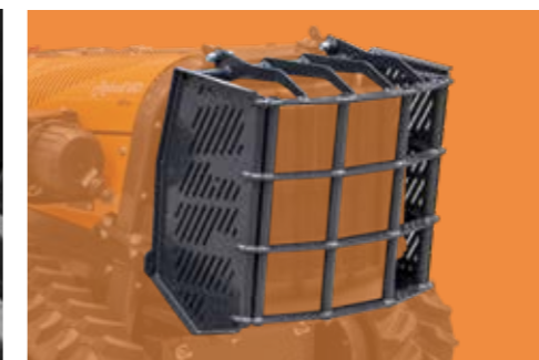
Steel radiator protection
