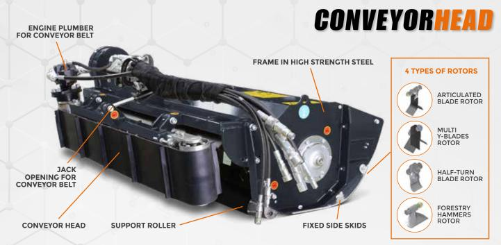
**CONVEYOR HEAD** is a cutting head whose frame is built in Domex steel. It rises from the experience of the project New Speed, well-established on the experience acquired over the years, Conveyor head differs from a traditional classic cutting head in the larger dimension of the output channel of residual cut material, creating the opportunity to install a conveyor belt (hydraulically operated) to avoid that residual vegetation falls immediately behind the cutting head.
