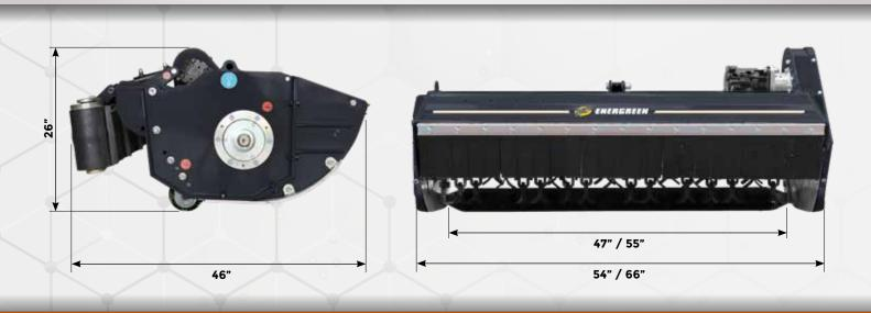
TECHNICAL DATA SHEET CUTTING HEAD WITH CONVEYOR BELT 47" / 59"
